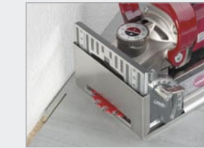
Expansion gaps (Saw blade Art. No. 132380 and slide shoe Art. No. 251058)
