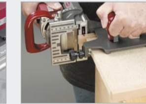
Trimming edges (Lamello Nova Art. No. 121280)
