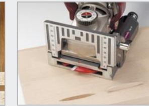
Wood repairs (Minispot cutter Art. No. 132217)
