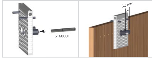
Rows of holes 5mm by moving the jig
