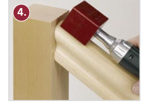
4. Connect the two parts with the MiniMag
