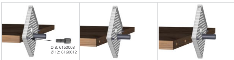
Rows of holes 8 and 12mm by moving the jig
